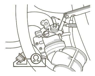
At point switch contacts close, Gap A must be between 0.05 - 0.10 mm (.002 - .004 in.)
