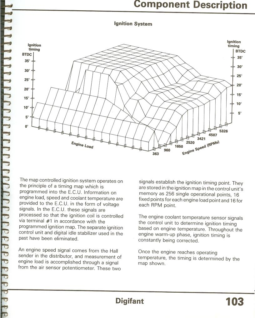
The map controlled ignition system operates on the principle of a timing map which is programmed into the E.C.U. Information on engine load, speed and coolant temperature are provided to the E.C.U. in the form of voltage signals. In the E.C.U. these signals are processed so that the ignition coil is controlled via terminal #1 in accordance with the programmed ignition map. The separate ignition control unit and digital idle stabilizer used in the past have been eliminated.
