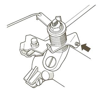
**Note:** Stop screw is set at factory and should not be moved. If screw position has been altered, check basic adjustment as follows:
