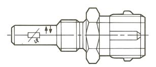
The coolant temperature sensor is a negative temperature coefficient resistor (NTC). The resistance signal it produces is used by the control unit to determine:
